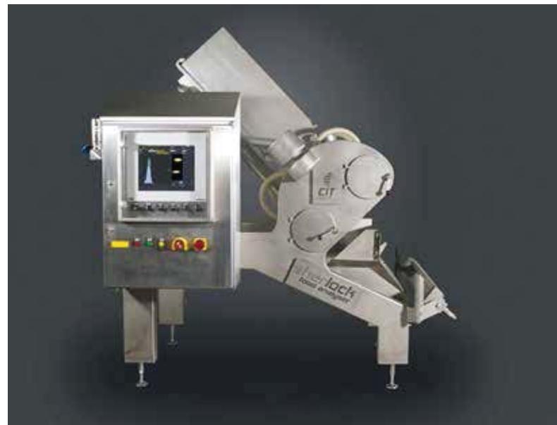
Inline food analyser based on IR spectroscopy
