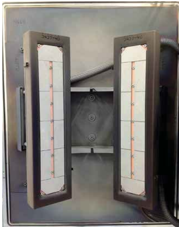
two titanium aluminum zircon square targets developed in the HIPERCUT project
